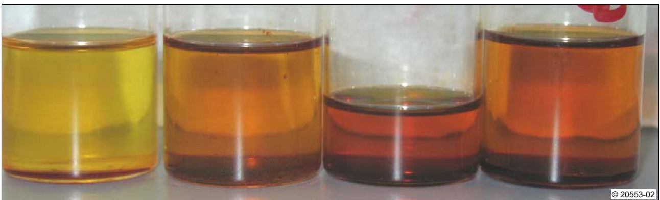
A2: Change in pure biodiesel in storage at 50 °C. Oxidised fuel components give biodiesel a dark colour.
