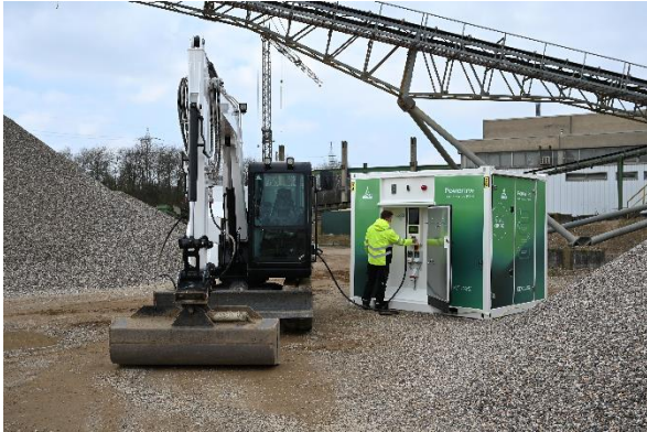
Caption: The electric-powered excavator can be charged rapidly using the PowerTree.
