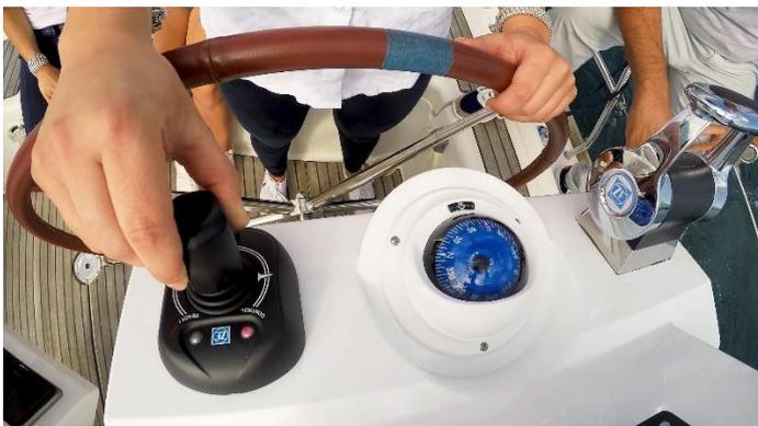
**Picture caption: Joystick docking enables the high-precision steering of the drive by joystick for docking maneuvers.**
