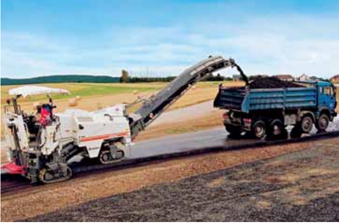
Wirtgen cold milling machine W1000F with 6-cylinder 1013 series engine.
