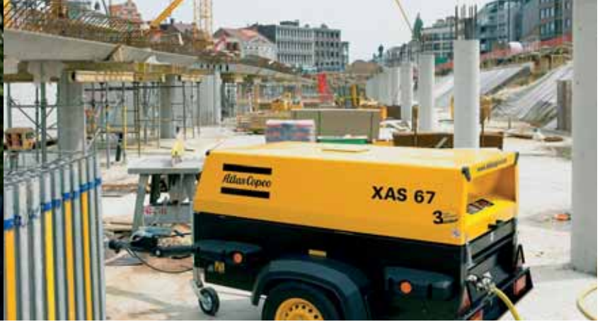
Atlas Copco compressor XAS 67 with 3-cylinder 2011 series engine.
