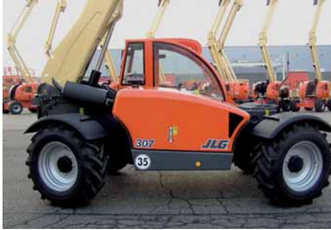
JLG telescopic handler 307 with 4-cylinder 2012 series engine.
